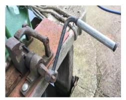
This is a windlass. Used on the paddle gear on the locks. It has two sizes of squares for different canal systems.
