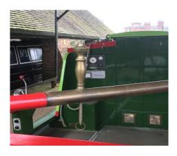
This is called tiller pin. Its used to anchor the brass tiller onto the swans neck. (looks like an 'S')
